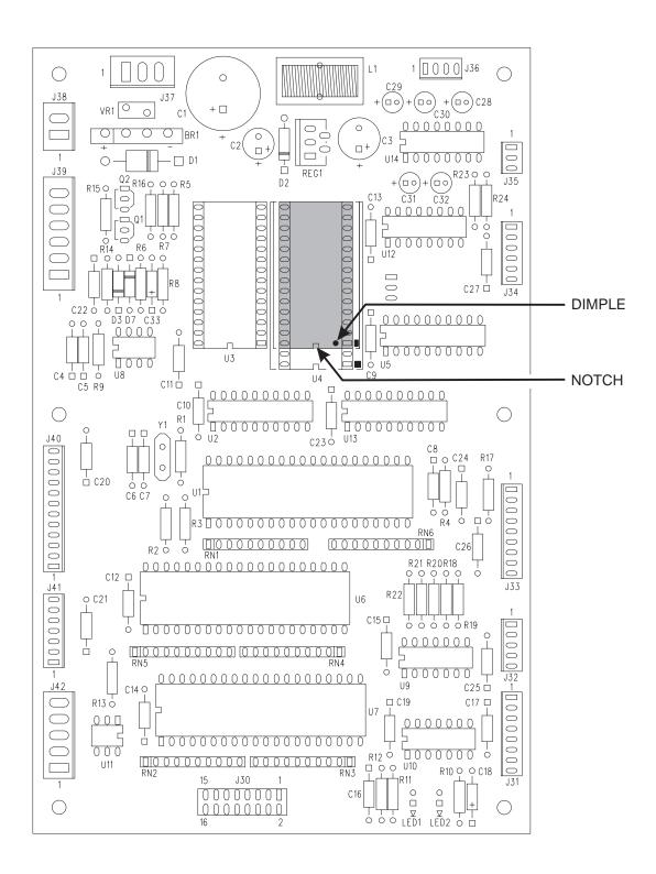
Figure 6. Controller Card Showing the Location of EPROM U4
